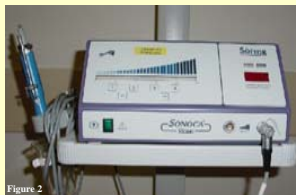
Figure 2 The SONOCA 180 was used to produce the sonication. Fluid normally flows through the tip to give the sonic waves a medium through which to travel. It also provides cooling for the tip.
