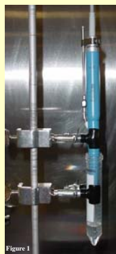
Figure 1 This is the basic set-up for our model. The conical tube was put into an ice bath to prevent overheating.
