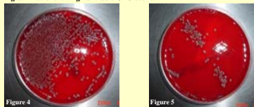
Figure 4 and 5 show the difference between an untreated plate and a plate exposed to 40 seconds of sonication in one of our preliminary tests.
